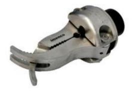
3-Finger Manipulator Jaw is the first choice for the vast majority of ROV Operators around the world. The 3 fingered manipulator jaw is intended as a hydraulically operated tool for attachment to a Schilling Robotics work-class ROV manipulator arm. The product is ideal for ROV operations where a combination of precision, flexibility and strength are required.
