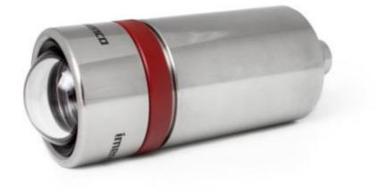
The Imenco Thresher Shark housing is constructed of titanium with a scratch and an impact resistant glass dome, and depth rating of 6.000msw. High Definition video: All major HD and SD video resolutions are supported e.g.:1080p/30,1080i/60,720p/60,720p/50.
