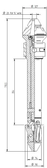
Lifting anchor measurements shown on figure above.
